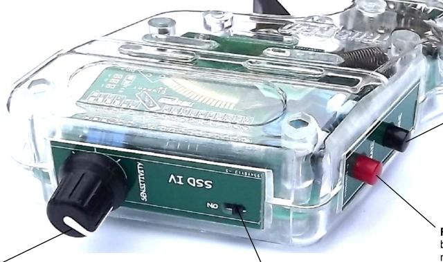
**Sensitivity knob** - turn left (anti-clockwise) for more gentle acceleration. Turn right (clockwise) for faster acceleration.
